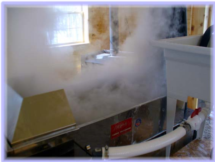
Close-up picture of steam from pan: "Water evaporates at a rapid rate from the Leader stainless steel pan, concentrating the sugar within the sap."
